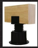
are spaced to accept 45mm timber and are grooved to allow easy penetration of fixing nails or screws. One 30mm galv or stainless (as required) nail or screw should be used on each side of the Timber Top® Spacings of Timber Tops® should be in accordance with NZS3604 2011 joist spans.(see section 7) to suit the size of the timber being used.
